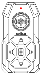
Blinking red Not connected
