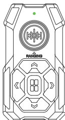
Blinking green Connected with device
